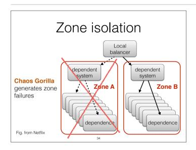
Netflix uses three zones in each region to limit the consequences of firmware failures, certain serious software bugs, power failures, and severe network failures. The zones correspond to different data centres. Note that the load balancer is a single point of failure.
