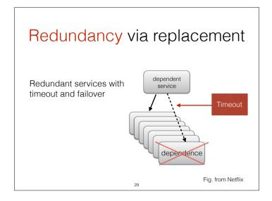
Micro-services are designed in to allows multiple instances to run behind a load balancer. If one instance goes down, then the calling instance can simply connect to another instance. An instance failure is often due to hardware error or network failure.
