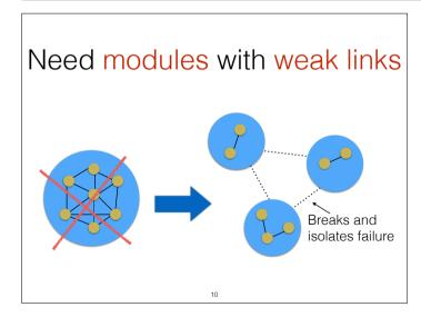
While the concept of "modules" is both well understood and much used, the concept of "weak links" is much less understood and used. Later, we'll discuss how the circuit breaker pattern realizes "weak links."
