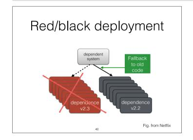
Use enough copies of new code in an auto-scaling group to carry the load. Keep the old code to ensure that we can handle peak load if there is a problem with the new code.
