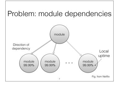
The figure illustrates module dependencies in a monolithic solution.
