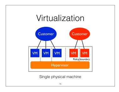
A **hypervisor** is computer software that runs Virtual Machines (VMs). Each VM is guest machine. The hypervisor presents the guest Operating Systems (OSs) with a virtual operating platform and manages the execution of the guest OSs. Multiple instances of different OSs may share the virtualized hardware resources.
