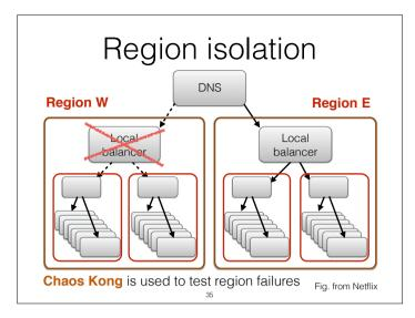
DNS (Domain Name Server) splits traffic load i two halves. To handle infrastructure failures, Netflix uses multiple regions and switch users to a new region when needed.
