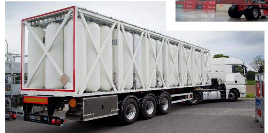
500 bar gas transport module (photo: Linde AG)
