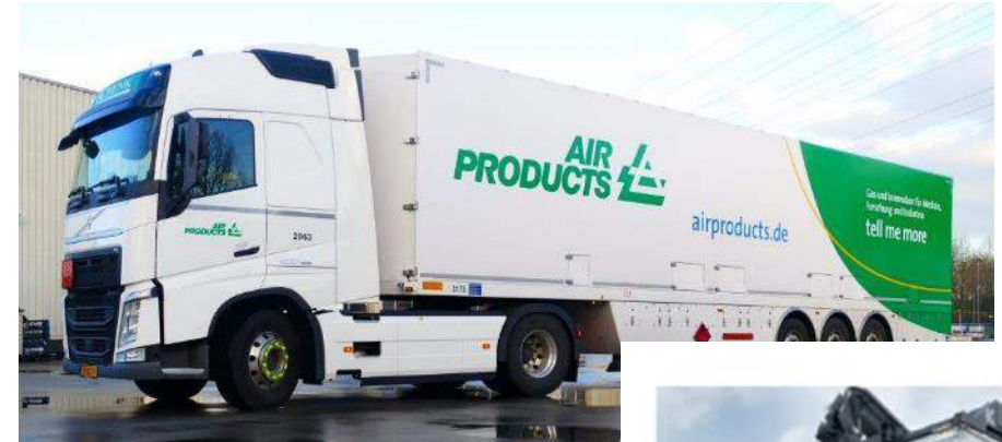
300 bar gas transport module (photo: Air Products)
